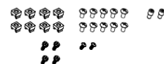
Fixing nut X 8, M6 screw X 10, M6 stud X 2, M4 screw X 4, M3 screw X 2
