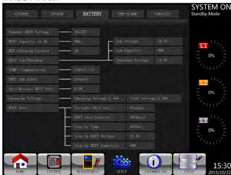
Battery Setup Screen
