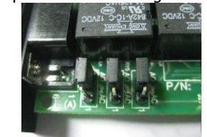
Fig. 7 Jumper setting for ACTIVE OPEN
