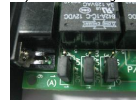
Fig. 6 Jumper setting for ACTIVE CLOSE
